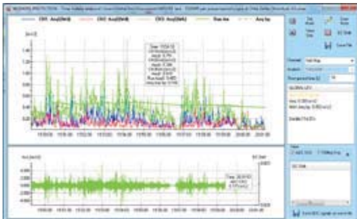
NS1 "Workers Protection" vibration module: vibration exposition evaluation, X, Y, Z axes time histories analysis. Vibration signal DC shift analysis.
