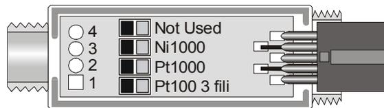
Before welding, pass the probe cable through the fairlead and gasket. Weld the temperature sensor wires as shown in the table:
