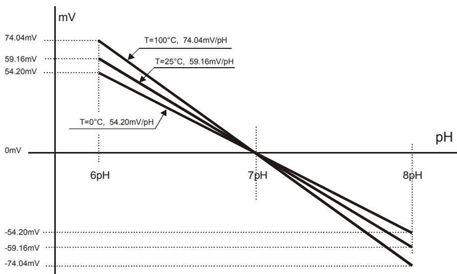
When a temperature probe is present, the instrument automatically applies the ATC automatic temperature compensation function. To disable it, the temperature probe must be disconnected. If the temperature probe is not present, and the correct value is not entered manually, the extent of the error committed in pH measurement is proportional to temperature and pH value itself.
