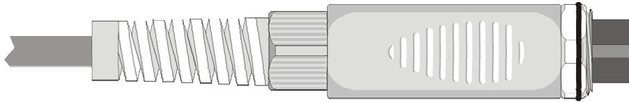
Make sure the cable is not twisted while you are screwing the fairlead. Now the probe is ready.
