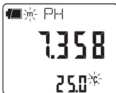
To manually change the compensation temperature press °C/°F once: the indicated temperature value starts blinking. Select the desired temperature value by using the arrows and confirm with ENTER. The display stops blinking, and the temperature displayed is used for compensation. To change the unit of measurement between °C and °F, it is necessary to press twice the °C/°F key.
