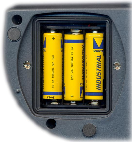
**After replacing the batteries, the menu parameters must be set again.** To go to the next item press ENTER; to return to measurement mode, press MENU.
