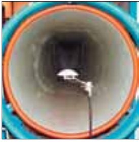
Static port put in front of the wind tunnel
