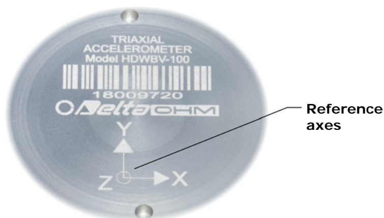
Fig. 4.1: Reference axes of the accelerometer
