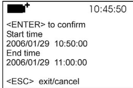
9. Press **ENTER** to confirm or **ESC** to exit without enabling the automatic start: In both cases, you will return to the **LOGGING** menu.
