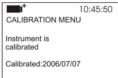
5. Press **ENTER** or **ESC** to go back to the main menu: you cannot change anything: **only Technical Support can calibrate the instrument.**
