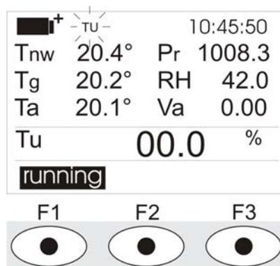
After few seconds the **TU** symbol will disappear, the **running** message will be replaced by **start** and the turbulence intensity value will be displayed.
