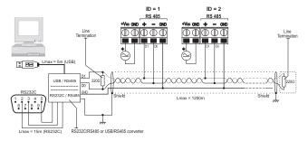
Line termination must be set at the two network ends. To polarize the line during nontransmission periods, resistor are connected between signal and power supply lines. The maximum number of devices that can be connected to the (Bus) line RS485 depends on the load characteristics of the devices to be connected.
