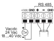
Thanks to RS485 output, several instruments can be connected to form a network. The instruments are connected in a sequence through a shielded cable with twisted pair for signals and a third wire for the ground.
