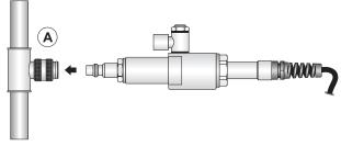
To connect with quick coupling, you can use one of the standard ¼" couplings provided. Other couplings than those supplied can be used, provided that they have a G ¼" thread on the side that fits into the probe.
