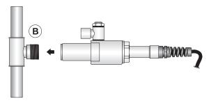
For the connection by threaded coupling, the connection must have an external G ¼" thread on the side which will be placed in the probe. The connection must be airtight. When installing or removing the probe, it is necessary to depressurize the system.
