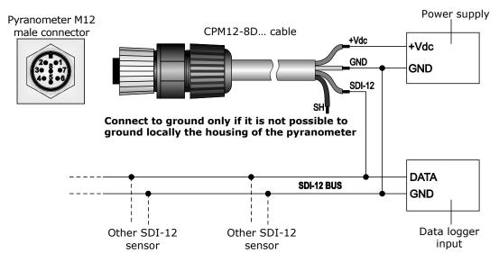
Fig. 4.5: LPPYRA03S12 connections
