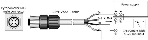
Connect to ground only if it is not possible to ground locally the housing of the pyranometer
