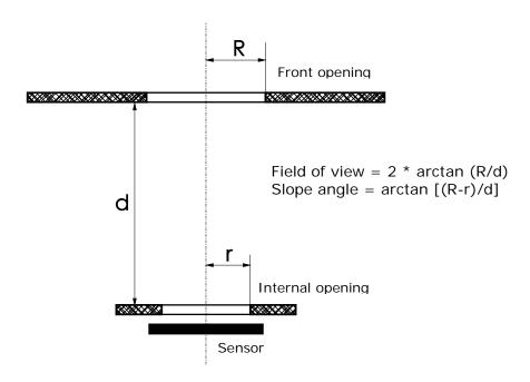
Fig. 2.2: field of view and slope angle
