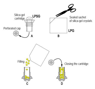
Fig. 3.1: filling the silica-gel cartridge
