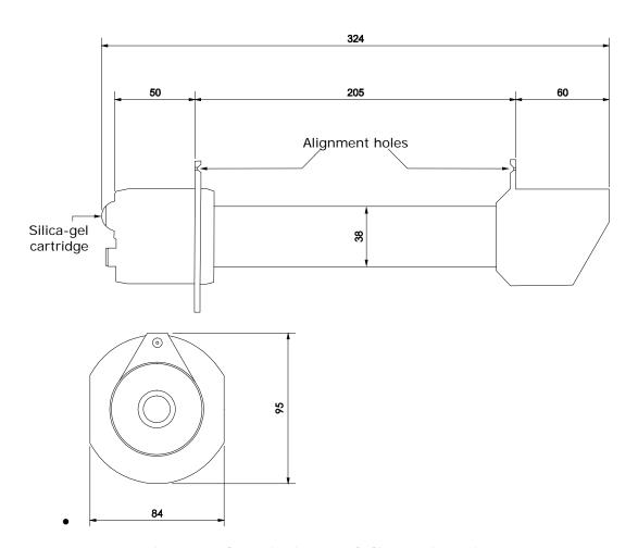
Fig. 3.2: description and dimensions in mm
