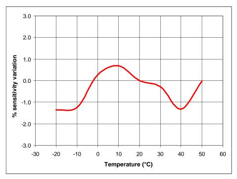
Fig. 2.1: % variation of sensitivity of the LPPYRHE16 pyrheliometer with regard to sensitivity at 20 °C in the temperature range from -20 to 50 °C
