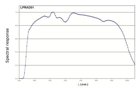
Probe calibration is carried out by using 577/579 nm lines of a Xe-Hg lamp, filtered through a special interferential filter. The temperature has a negligible influence on the spectral response of the probe.
