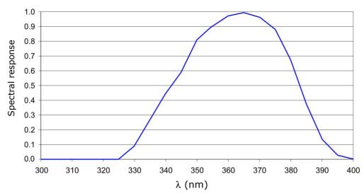
The calibration is performed by reference to our primary standard with monochromatic light at 365 nm obtained separating the emission line of a Xe-Hg lamp with an inferential filter. To get best performances from your LPUVA01 it is strongly recommended that the calibration be checked annually. The temperature has a negligible influence on the spectral response of the probe.
