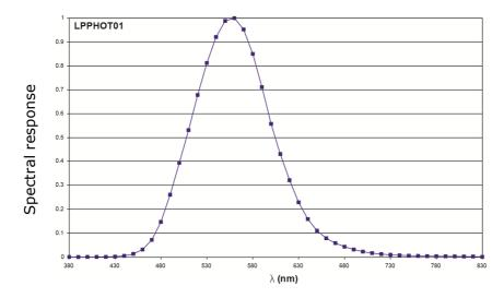
The calibration of the probe is performed by comparing it to a luxmeter calibrated by a Primary Metrological Institute. The calibration procedure follows the CIE publication No 69 (1987) "Method of Characterizing Illuminance Meters" and Luminance Meters" and is carried out by illuminating the probe with a standard illuminant A.
