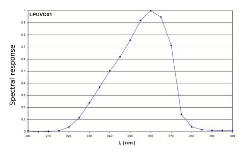
The probe calibration is carried out by measuring irradiance coming from an Hg lamp at 254 nm.
