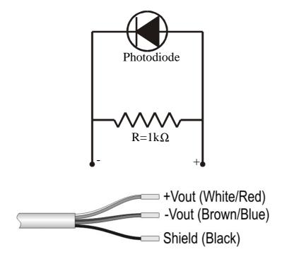
To obtain a reading precision of 1% of the difference in potential at the ends of the resistance, the probe must be connected to a digital multimeter with input resistance > 100  $k\Omega$
