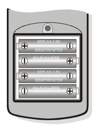
After replacing the batteries, the date, time, baud rate, type of probe, printing interval, logging parameters must be set again: in order to simplify the operation, on insertion of the new batteries the instrument turns on automatically and requests these parameters in sequence. To go to the next item press ENTER; to return to measurement mode, press MENU.
