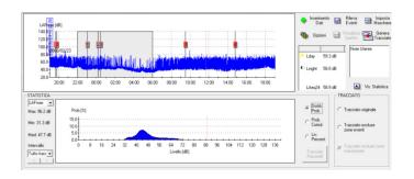
Daily charts and events table: daily processing allows to detect events on threshold conditions and to divide them over reference periods in a tabular format. Events detection function allows to serch for impulses in the time profiles. Statistic is available both in graphic and numerical format as probability distribution, cumulative distribution and percentile levels.
