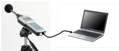
Cable connection RS232 or USB
