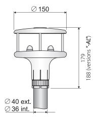
Air speed Air direction Pressure (optionally)
