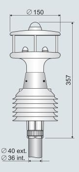
Air speed Air direction Temperature Relative Humidity Solar radiation Pressure (optionally)
