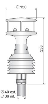
Air speed Air direction Temperature Relative Humidity Pressure (optionally)
