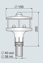
Air speed Air direction Solar radiation Pressure (optionally)
