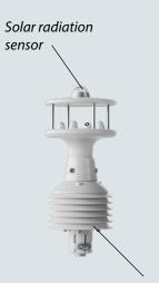
Temperature and relative humidity sensors with solar radiations protection shield
