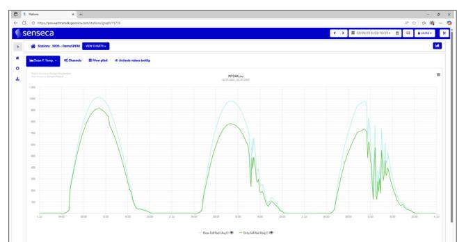
Solar radiation signals from 'clean cell' and 'dirty cell' collected by MDFS (displayed using webtrans-w4k application)
