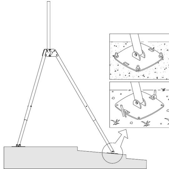
The flanges of the tripod can be fixed on a floor with screws or on the ground with pegs.
