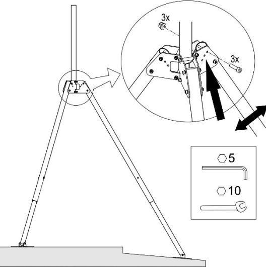
Secure the legs to the central block of the tripod.
