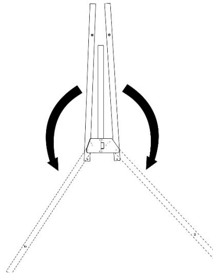
Open the tripod by turning the three legs.
