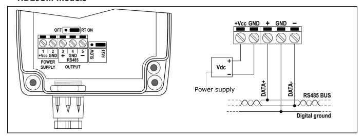
Before connecting the transmitter to the RS485 network, set the address and the communication parameters, if different from the factory preset (see "Configuration" chapter). The output is not isolated.
