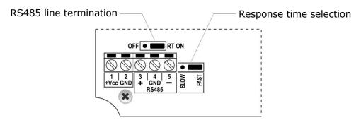
The "RT" short jumper allows inserting an RS485 line termination built into the transmitter.
