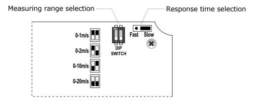
The dip switches allow the configuration of different speed ranges to be associated with the analog output:
