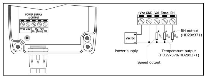
The load resistance  $R_L$  varies according to the type of analog output:
