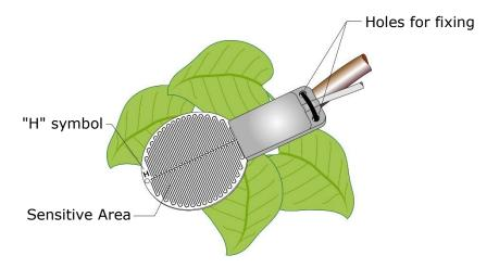
The sensor should be inclined at about  $30 \div 45^{\circ}$  with respect to the ground, so as to prevent the stagnation of condensation or rainwater on the sensitive surface and simulate the real condition of the leaf type of the cultivation under examination.
