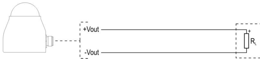
Fig. 4.5: LPPYRA-Lite connection diagram
