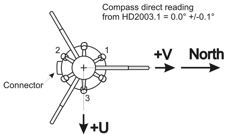
HD2003.1 Ultrasonic Anemometer
