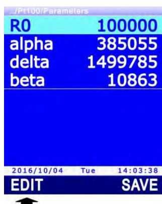
Fig. 13.2.3: parameters for temperature calculation equation
