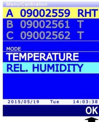
Fig. 13.3.1: selecting the sensor to be calibrated
