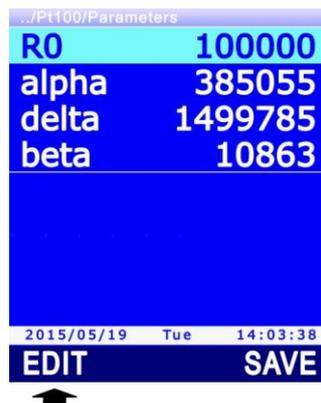
**Fig. 13.1.3: parameters for temperature calculation equation**
