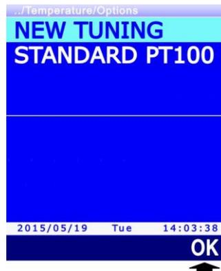
Fig. 13.3.2: types of calibration for the temperature sensor
