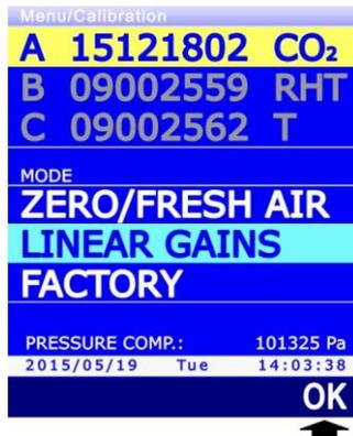
**Fig. 13.5.1: calibrations for CO<sub>2</sub> probes**
