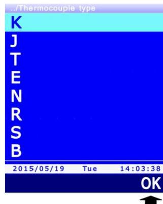
**Fig. 13.2.1: selecting the type of thermocouple**
