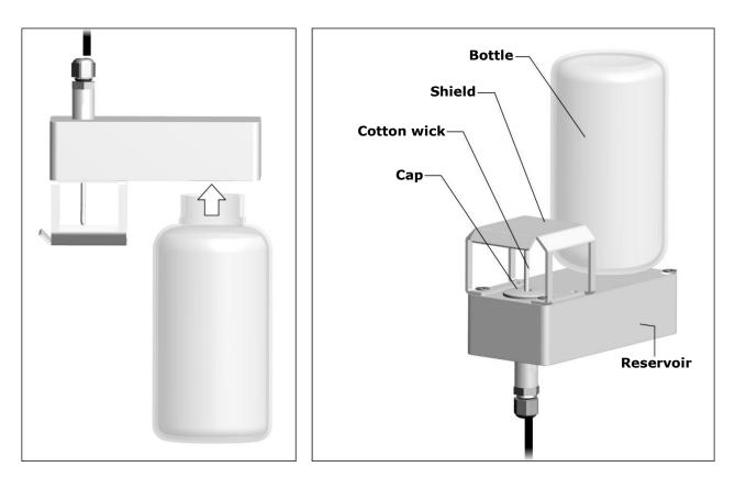
For measurements in presence of solar irradiation, use the protection shield from solar radiations. *Note*: over time the cotton wick tends to calcify (harden): it must be replaced periodically.
