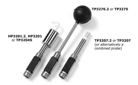
Probes necessary for **PMV/PPD** indices measurement:
