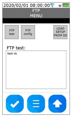
The configuration of the FTP connection can be entered using the virtual keyboard of the instrument or it is possible to load the configuration from a text file present in the instrument memory.
