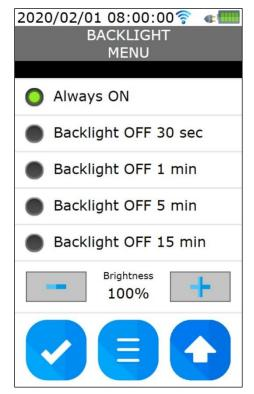
Use the +/- keys to adjust the display brightness. The lower the display brightness, the longer the battery autonomy will be.
