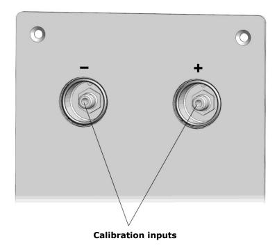
The differential pressure zero calibration is also possible via the Modbus Coil register with address 72 (see chapter 11).
