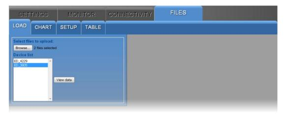
Press the *Browse...* key and select the files to be imported (multiple files can be selected). The instrument corresponding to the imported files appear in the *Device list*: select an instrument and press *View data* to display the data.
