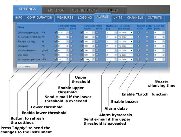
If the *Buzzer Latch* option is enabled, the buzzer continues to sound even after the alarm condition has ceased. The *Alarm ack* field allows silencing the buzzer for the set number of minutes.
