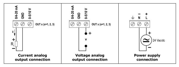
Current outputs max. load 500  $\Omega$ ; voltage outputs min. load 10 k $\Omega$ .
