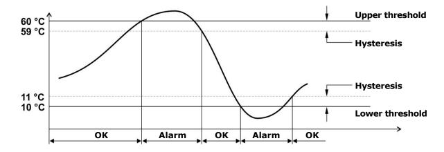
The alarm is generated after the set delay time or immediately if the "no delay" option is selected (default). If the alarm condition disappears before the delay time has elapsed, the alarm is not generated.
