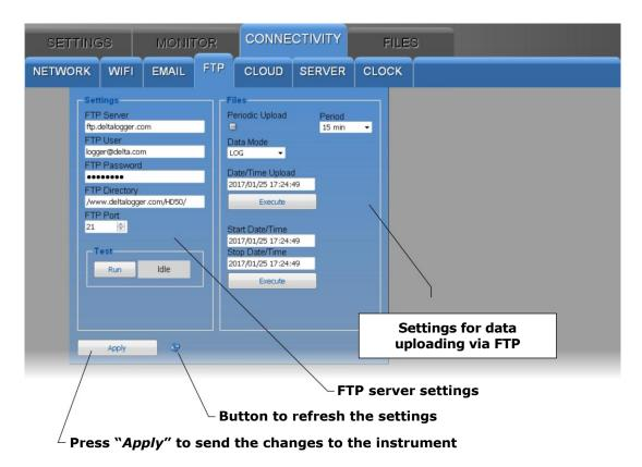
The Settings section of the FTP panel consists of the following fields:
