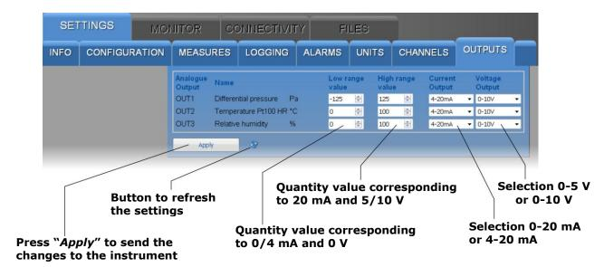
The three analog outputs are associated with the first three quantities of the list of selected quantities in the *CHANNELS* panel.
