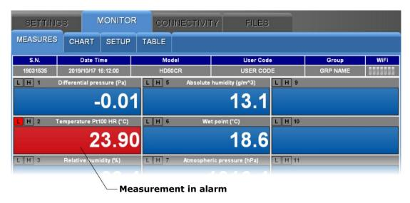
The measurements in alarm are highlighted with a red background. The  $\bf L$  and  $\bf H$  symbols indicate whether the lower (L) or higher (H) threshold has been exceeded.
