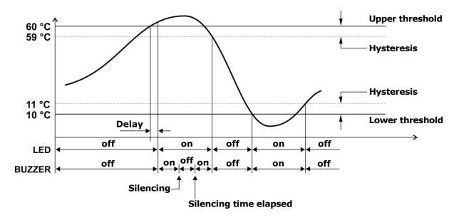
The following example shows the silencing of the buzzer with *Latch* option enabled.
