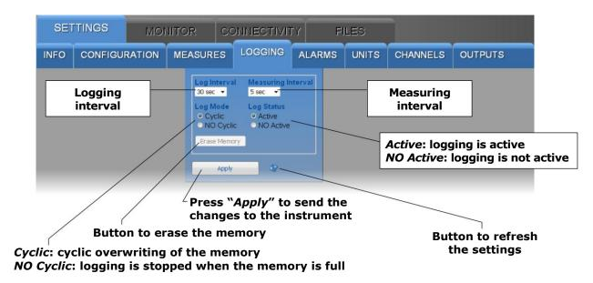
If the logging interval is greater than the measuring interval, the average of the measurements acquired during the logging interval will be stored.
