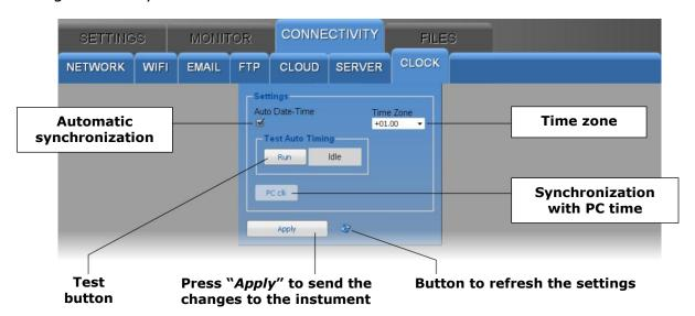
Select the *Auto Date-Time* check box to keep the clock synchronized with a NIST reference server (if the instrument is connected to the local network and the Internet connection is available). Press the *Run* key to check the automatic synchronization; the box next to the *Run* key displays the progress of the test and the final result.
