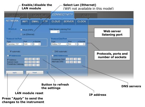
*Note*: if the instrument IP address is changed, the new address must be entered in the web browser to connect to the web server.
