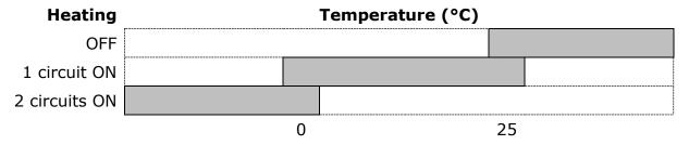
The exact temperature at which to activate the heating can also depend on other climatic factors. For example, the probability of dew forming on the dome is affected by whether the climate is dry or humid. Therefore, the exact activation temperature should be adapted to the place of installation.
